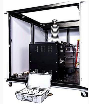
Control panel is mounted on 6' cabinet or a remote field box is available
