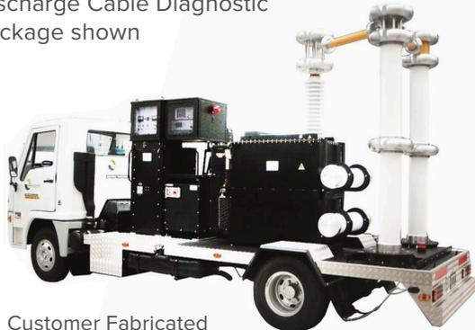
Customer Fabricated Test Truck
