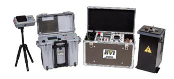
☐ The VLF & VLF E Series 0.1 Hz. hipots are for testing loads of very high capacitance, like MV/HV power cables and large rotating machinery that would require hundreds of kVA of test power at 50/60 Hz. Very Low Frequency (VLF) AC Technology is available in model sizes from 30 kVac - 200 kVac, able to perform testing of loads from  $0.1 \mu F - 50 \mu F$ . IEEE400.2-2013 & IEEE433-2012 apply. VLF TD and PD testing available.
