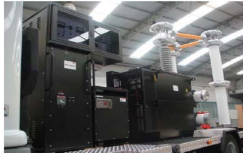
220 kv VLF-200 HVCD mobile unit, with Tangent Delta/Partial Discharge test capacity (INDUCOR INGENIERIA S.A.)
