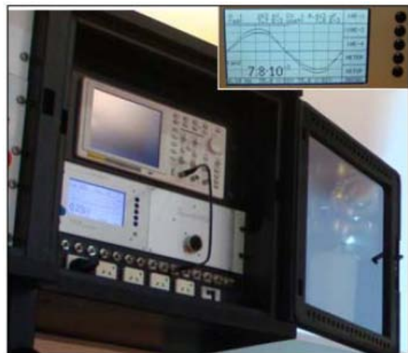
PD measurement panel of the VLF-200 HVCD system
