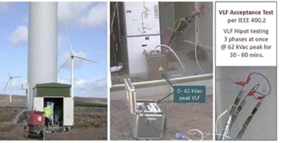
Cable system is new but needs VLF Withstand test to find faulty workmanship on splices and terminations and possible cable installation damage. Tan Delta and Partial Discharge testing are not needed. VLF It!
