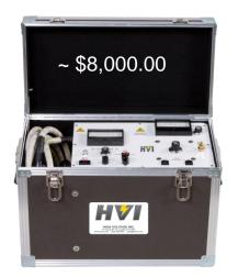
0-50 kVac @ 3 kVA, 50/60 Hz. Can test only ~50' of 15 kV cable = .0026 µF of load
