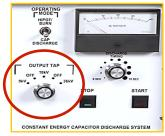
You can thump a cable at only 9 kV @ 3200 Joules, find the fault, but without severely over-stressing the entire cable system, and adjacent cables, with extreme voltages.
