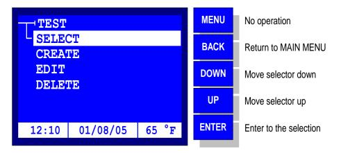
The Test Submenu is displayed upon the TEST Selection from the Main Menu, The possible selections are the following:
