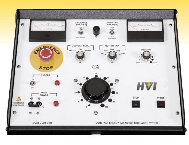
Main Power On Cap Discharge Mode Select Output Tap Coupler in Radar mode **Press Start** Raise to desired Voltage
