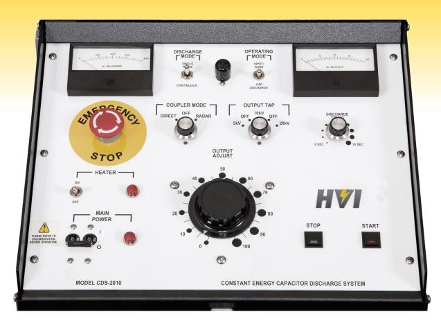
Main Power On Cap Discharge Mode Select Output Tap Coupler – Direct mode **Press Start Raise Voltage** Let caps charge Discharge Mode - Continuous
