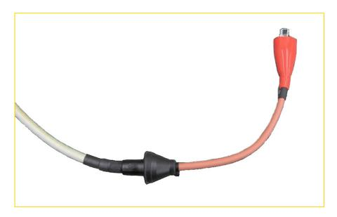
It is important to treat the entire unshielded (pink) part of the cable as if it was at high voltage. Never lay the pink insulation across a grounded surface or there is danger of insulation puncture. Also note that the white part of the cable is a plastic jacket layer over the grounded cable shield. Do not lay the pink part across the white part either.
